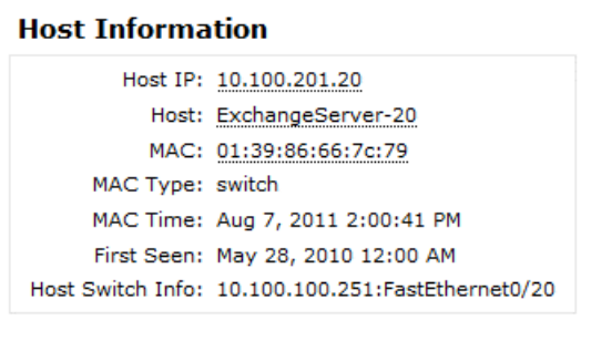
Figure 6-1. MAC and Host Switch Information Displayed as a Result of Switch Port Discovery
