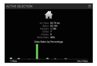
The **Active Selection** legend displays the related data to the center of the multi-layered pie chart. This data will change as the user drills down through layers. It displays total airtime, byes, number of packets, SSIDs, clients, and retry rate percentages. Below this information is a bar chart displaying the percentage of clients active at each detected data rate.
