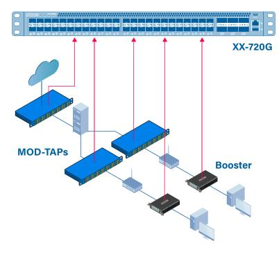
To access traffic reliably and with high performance, fiber TAPs were used as the first bricks of the network architecture infrastructure.
