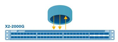
All the traffic coming out from the Profitap XX-720G Network Packet Brokers is fed into the <u>Profitap X2-2000G</u>: a Next-Generation Network Packet Broker (NGNPB) with a total throughput of 2 Tbps. The Profitap X2-2000G provides aggregation, replication, powerful filtering, and load balancing in very high bandwidth port monitoring and analysis scenarios.
