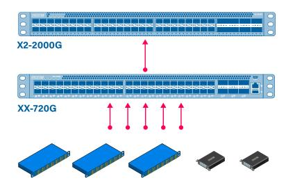
After accessing the network traffic with Fiber and Aggregation TAPs, the traffic needed to be monitored and optimized. In order to aggregate and distribute the right traffic between the TAPs and X2-2000G in a cost-effective way, multiple XX-720G high-density Network Packet Brokers were selected as the first layer of aggregation.
