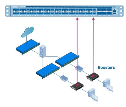
In order to access copper network links of up to 1 Gbps, the Profitap Booster has been placed at key points.
