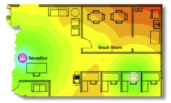
**Regular, ongoing surveys**: Maintaining high performance and coverage requires regular "check-up" surveys. New users, new equipment, site expansion, neighboring WLANs, and other factors can adversely affect your WLAN. It should be monitored on a regular basis.
