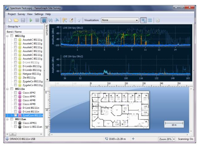
The spectrum pane is similar to the one you can see in *Chanalyzer*, a spectrum analysis application by MetaGeek that comes with Wi-Spy. By default, the spectrum pane displays one or two planar spectrum graphs for single- and dual-band Wi-Spy models, respectively.
