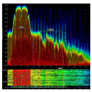
Chanalyzer is designed to bring simplicity and power to the process of wireless troubleshooting. It combines Wi-Spy's ability to read raw RF data with your computer's built-in Wi-Fi card to show you how environmental Wi-Fi saturation and non-Wi-Fi transmitters are affecting your network. Chanalyzer is capable of displaying activity in the 2.4 GHz band, 5 GHz band, or both simultaneously if using Wi-Spy DBx or a Cisco access Point.
