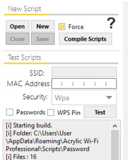
In the script testing section, you can specify the script test parameters to validate they are working correctly. Access point, SSID, MAC and security type fields should be completed in order to run the test. You need to specify whether you are testing passwords or WPS PINs. Finally, you need to click on the Test button to start a new test.
