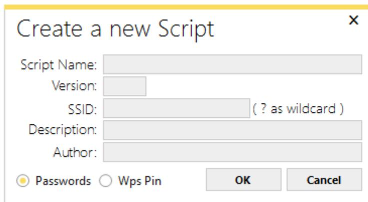
To make scripting easier, when you create a new script, a window requesting the main details is displayed to help generate a script template, which will be ready to inject code into the Generate function.
