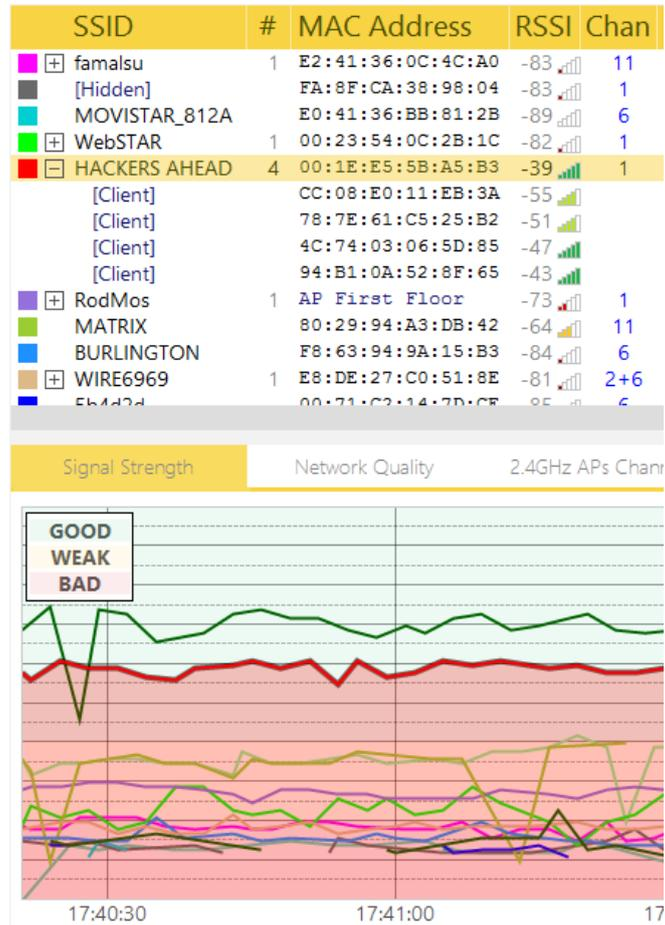
Each row represents an access point, and each column includes information such as signal strength, SNR, MAC address, security options, etc.
