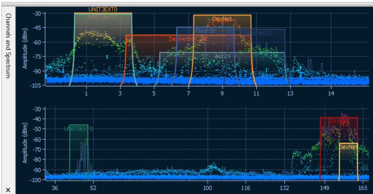
The spectrum pane is similar to the one you can see in *Chanalyzer*, a spectrum analysis application by MetaGeek that comes with Wi-Spy. By default, the **Channels and Spectrum** pane displays one or two planar spectrum graphs for single- and dual-band Wi-Spy models, respectively.
