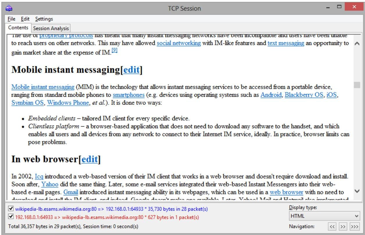
In HTML display mode, HTML pages typically do not include inline graphics, because in HTTP protocol images are transferred separately from HTML data. To view the images, it is usually necessary to navigate to the next TCP session. A sample HTTP session that contains image data displayed in HTML mode is shown below:
