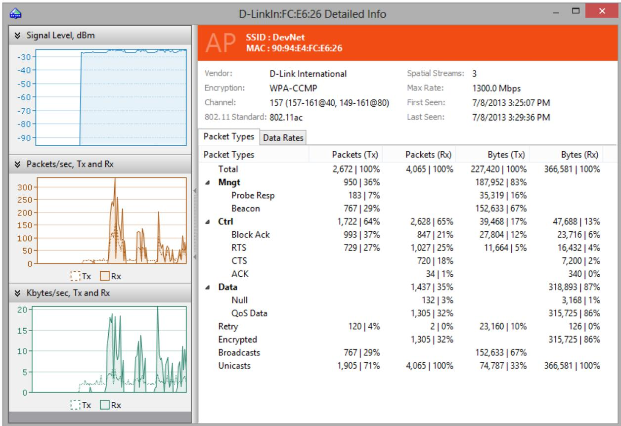
The top pane displays the type, MAC address, and SSID of the selected node, followed by other key details, such as channel, first seen and last seen times, etc. This pane uses the same color that is used to display the selected AP on the **Channels and Spectrum** pane of the main application window.
