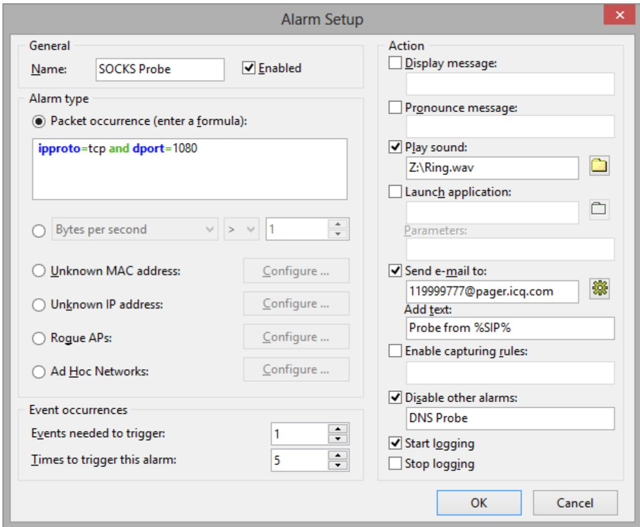
The **Name** field should be used for describing the alarm function. Check the **Enabled** box if you want the alarm that you are adding/editing to be activated once you have finished its setup. This check box is equivalent to the one shown in the alarms list. The **Alarm Type** frame allows you to select one of the ten alarm types:
