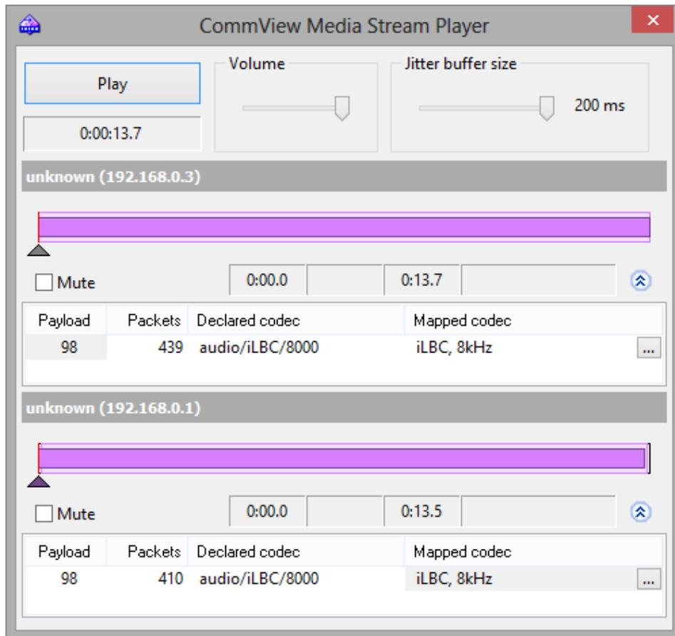
Click on the double-arrow button to have the application display more detailed information about the audio stream(s) and access to manual codec mapping. For each of the RTP streams you can:
