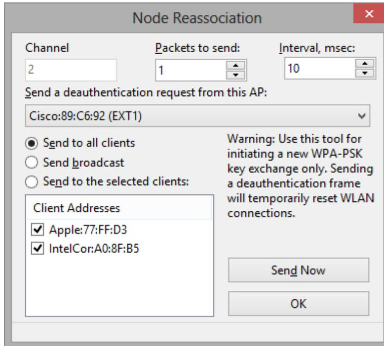
This tool simply sends a deauthentication request to the selected stations on behalf of the access point. This causes the stations to reassociate with the access point. The reassociation process usually takes a second and lets CommView for WiFi capture EAPOL packets necessary for WPA-PSK decryption. Do not use this tool unless you need to decrypt WPA-PSK traffic on your WLAN.
