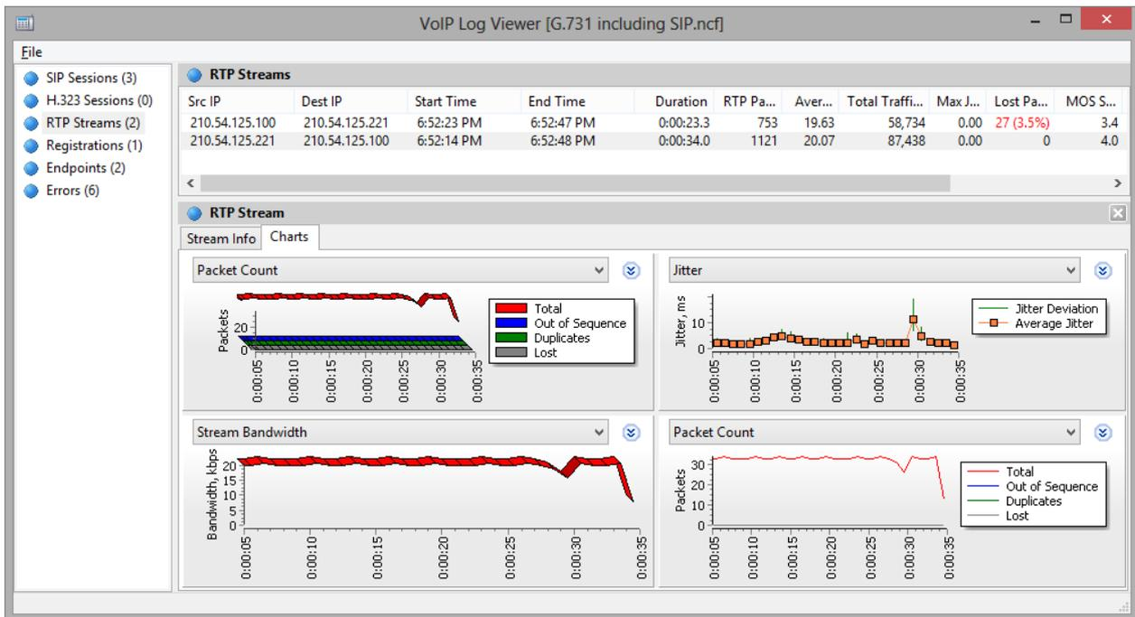
Up to four different charts for the selected stream can be displayed simultaneously, with the window interval from 5 to 60 seconds. Note that right clicking and dragging the graph will scroll it to the left or right respectively. The following chart types are available:
