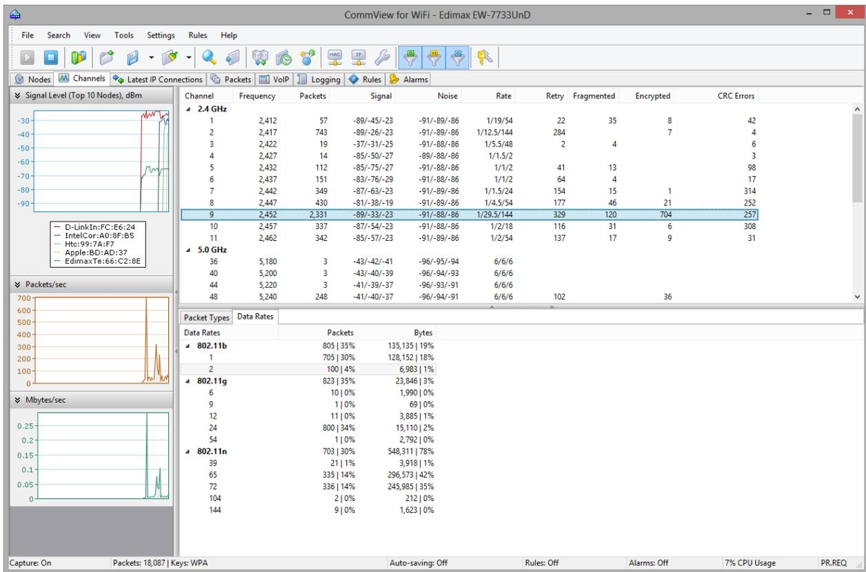
Because the 802.11 standard uses overlapping channel frequencies in the 2.4 GHz band, you might notice that even if your WLAN is configured to use only one channel, e.g. 6, you will still see non-zero values for the adjacent channels. Unlike 2.4 GHz channels, 5 GHz channels do not overlap.
