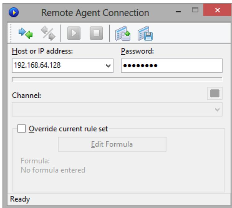
Click on the **New Remote Agent Connection** button to establish a new connection, or click on the **Load Remote Agent Profile** toolbar button to load a previously saved Remote Agent connection profile. A previously saved profile may also be loaded from the New Remote Agent Connection window.
