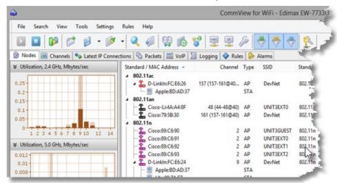
packet sniffer for 802.11 a/b/g/n/ac/ax networks.
