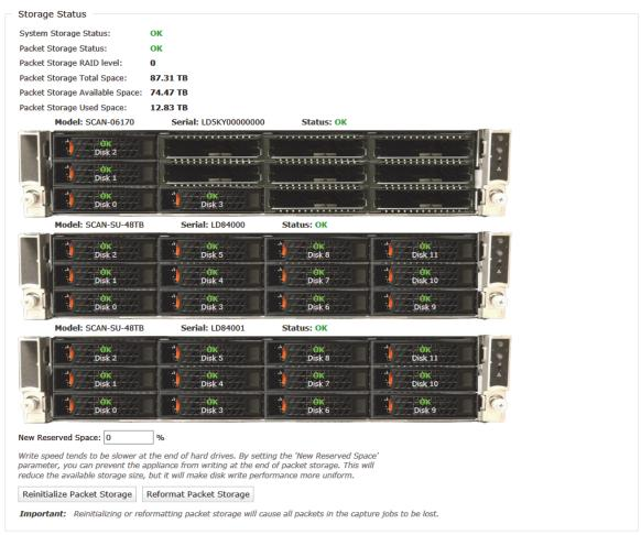
When a disk is failing or fails its status changes in the Storage Status information. The Fault LED on the disk drive is On. If enabled, a notification also is sent or logged, reporting a change in storage status.
