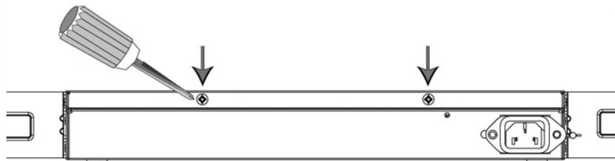
Figure 2-3. Removing the locking screws
