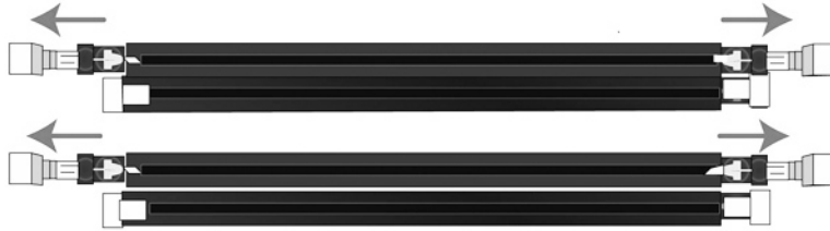
Figure 2-24. Accessing the memory modules
