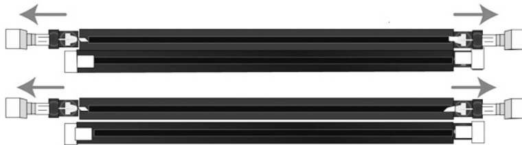
Figure 3-12. Accessing the memory modules
