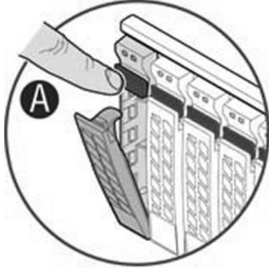
Figure 1-17. Releasing the disk drive
