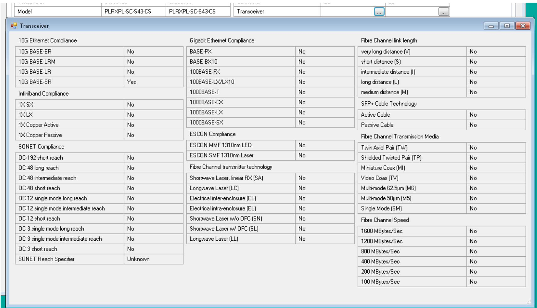
Figure 28: SFP+ Transceiver Details
